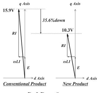
Fig. 3: Phasor diagram (N = 3000 min<sup>-1</sup>)
