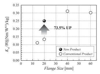
Fig. 8: Comparison of motor constant density
