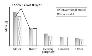
Fig. 4: Mass pallet analysis per component
